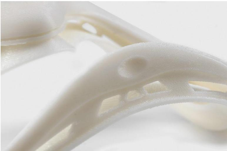
FDM parts tend to have visible layer lines and might show inaccuracies around complex features. This example was printed on a Stratasys uPrint industrial FDM 3D printer with soluble supports (machine starting at \$15,900).
